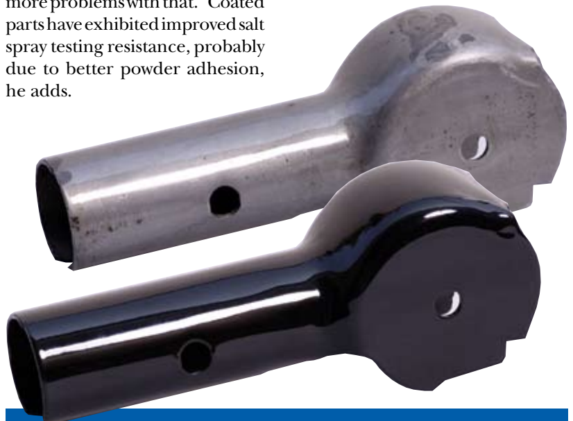
Microfinish receives parts in all conditions, from already clean to dripping with oil. Parts are shown before pretreatment and after powder coating.
